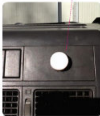
Audio-visible signal installed in the console of the truck
