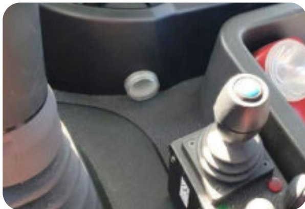
Audio-visible signal installed in the console of the truck
